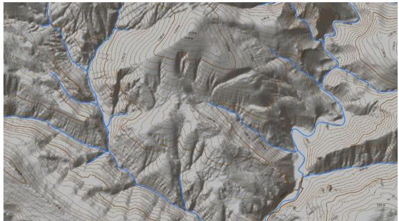
Hydrographic network obtained automatically from LIDAR DEM.
